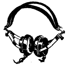
No. 3—A Head Set No. 3—A Head Set Permanently sensitive. Magnets exert 2 1/2 lbs. pull. Hard Rubber Ear Caps. Die Cast Aluminum Case, Nickeled Head Band with Swivel and Slide Adjustment. 11,000 ohms total impedance. PRICE $5.50
